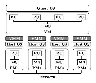
Figure 1: A virtual machine (VM) with four processors built on four single-processor physical machines (PMs). PU and MS denote a processor unit and a main memory (storage) unit respectively.
